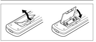
Open the lid of the battery compartment on the rear of the remote control unit, and insert the batteries, taking care to align the  $\bigoplus$  and  $\bigoplus$  polarities correctly.
